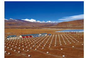
Tibet Air Shower Observation Array. Scintillation detectors are composed of approximately 800 units arranged over approximately 3.7 ha.
