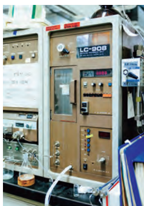
A device for purifying polymers Yokozawa has been using for more than twenty years. The nature of reactions can be determined by separately analyzing those high- and low-molecular-weight molecules.
